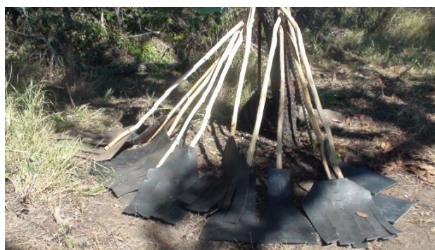
Plate 3: Fire beaters improvised by Mat South villagers from Conveyor belts
